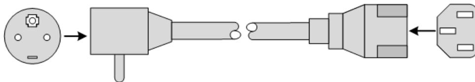
The AC power cable which meets American standard is composed of the American 3-pin plug and 3-pin receptacle connector, as shown in Figure 5-11.
