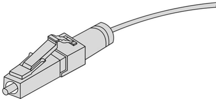
When connecting or removing the LC/PC fiber connector, align the fiber connector with the optical interface, and do not rotate the fiber. Note the following points:
