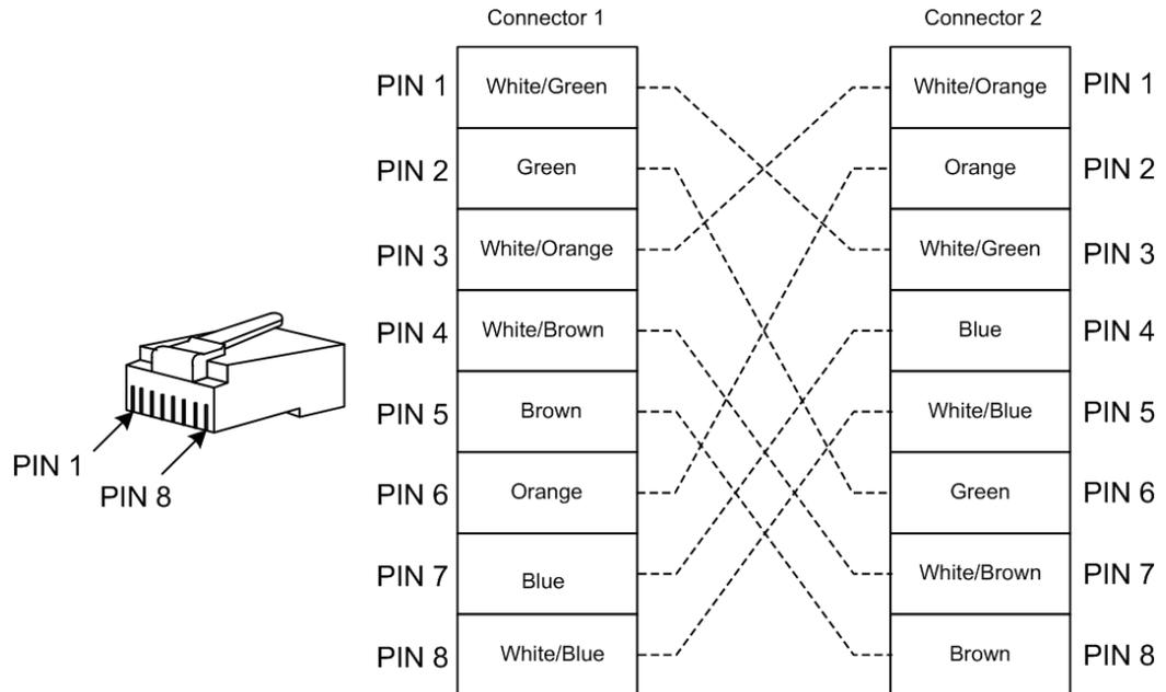
Raisecom provides the straight-through cable and 100 Mbit/s crossover cable which are only different in name. The straight-through cable is named as CBL-ETH-RJ45/RJ45-D while the crossover cable is named as CBL-ETH-RJ45/RJ45-X-D.
