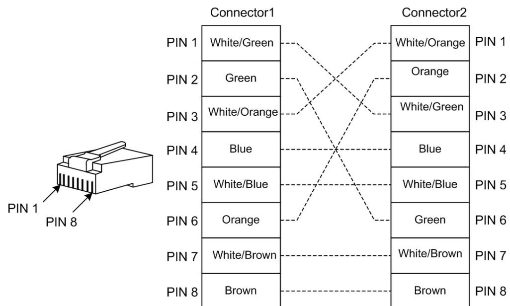
The 1000 Mbit/s crossover cable uses all 8 pins of the twisted-pair cable. The crossover is PIN 1 to PIN 3, PIN 2 to PIN 6, PIN 4 to PIN 7, and PIN 5 to PIN 8, as shown in Figure 5-5.
