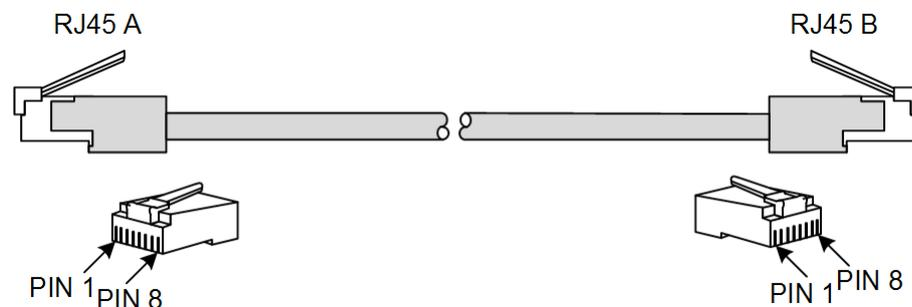
Figure 5-7 shows the appearance of the CBL-E1-RJ45/2RJ45 E1 balanced cable.
